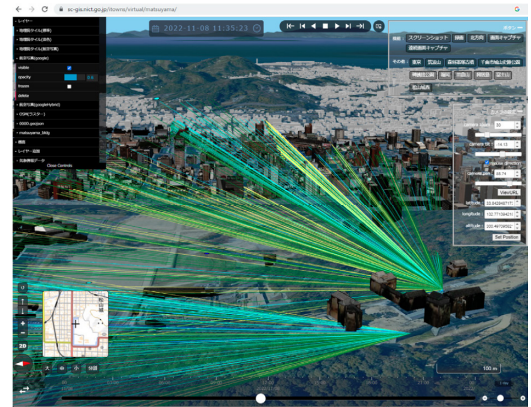
Fig.3 : Data visualization app example: Matsuyama City PLATEAU Building + LPWA (920 MHz) communications experiment visualization
