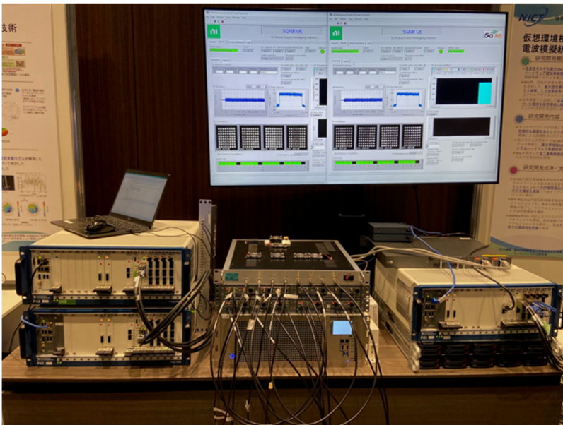
Fig.4 : Demonstration setup of SDR-based 5G NR system in symposium
